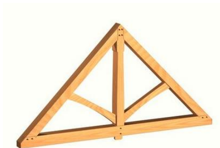
Figures 13 (left) and 14 (right) – Preliminary Sketch of Potential King Post Truss System Design (left); Image of a Basic King Post Truss from www.precraftedhomes.com (right)
