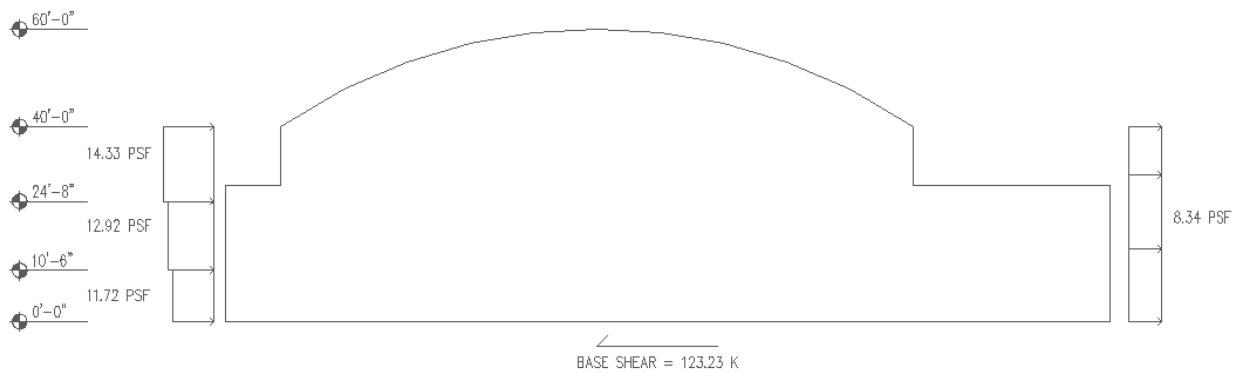
Figure 57 - Wind Loads on Entire Building (East/West)
